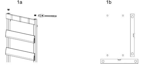
2. Using the drill and 8mm drill bit, drill into the marked positions then insert the wall plugs and tap flush to the finished wall surface.
