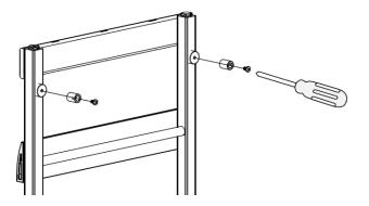
5. Align and push the rail brackets on the radiator onto the wall brackets secured to the wall. Secure the two together with the connecting screws provided (insert through the slot in the bracket) and tighten by the Philips screwdriver, be sure not to overtighten.
